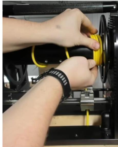
3. While holding your organized cable, pull the *tether* slack back through the *Levelwind Carriage* so there is no slack between the *Levelwind Carriage* and the *Drum*.
