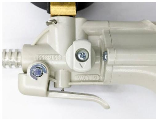
5. Pump the vacuum until the gauge reads 10 inHg [34 kPa] vacuum.
