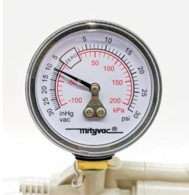
If the gauge reads below 9 inHg [31 kPa] vacuum after 15 minutes, you should check the following:
