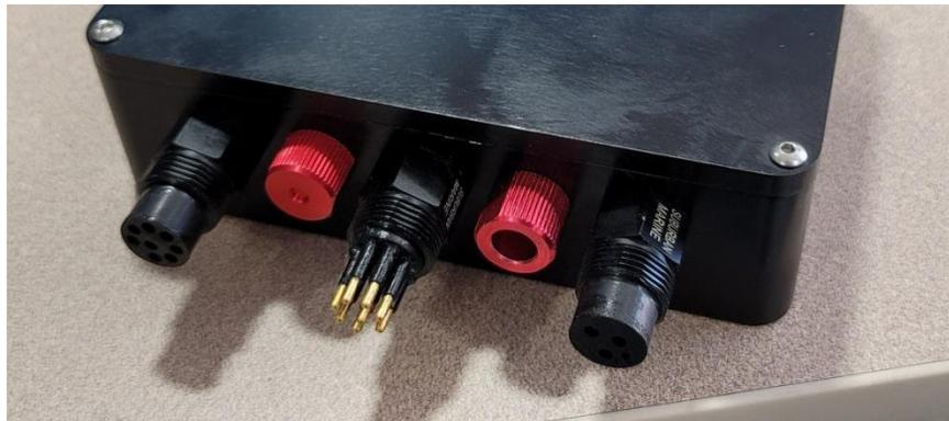
3. Insert the other vacuum plug into the Electronics Enclosure vent penetrator.
