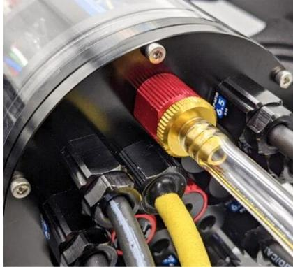
4. Turn the knob on the side of the vacuum pump so it is in the “VACUUM” setting.
