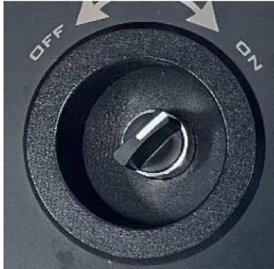
**Note: Following turning on power to the ROV, you should hear a series of beeps and whistles coming from the ROV. This confirms power is supplied to the ROV successfully.**
